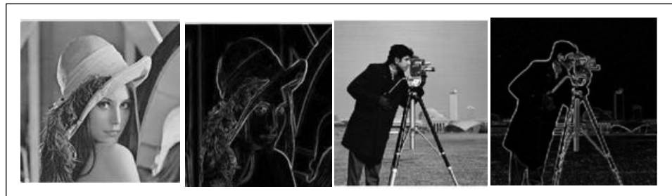
Figure 2.2.6: The application Sample of Prewitt operator on image
